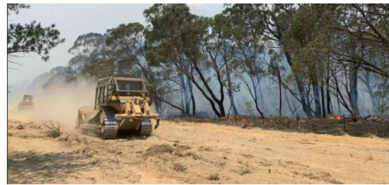
Heavy plant building a fire break south of Nerriga
